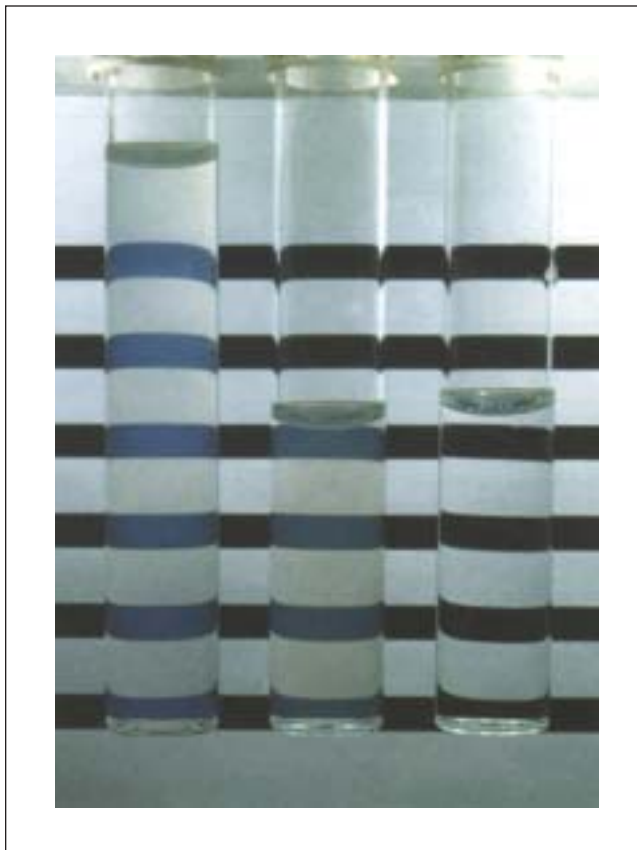
FIGURE 51: Comparison of the 0.5 McFarland turbidity standard with inoculum suspension
