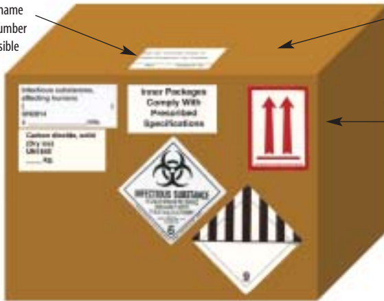
Figure E: Overpack with <50 ml infectious substance and dry ice
