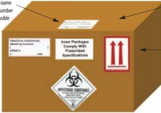
Figure C: Overpack with <50 ml of infectious substance
