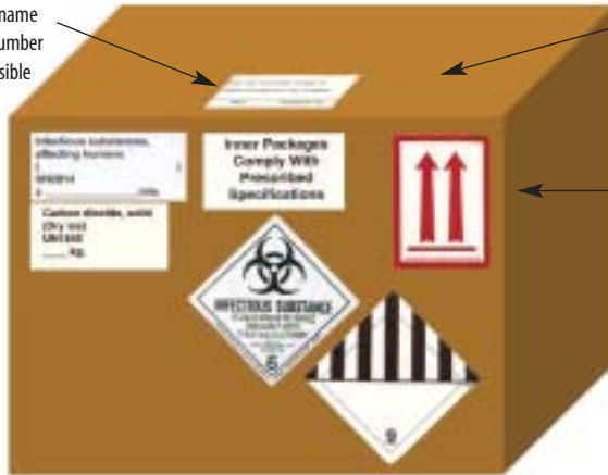
Figure F: Overpack with \geq 50 ml infectious substance and dry ice
