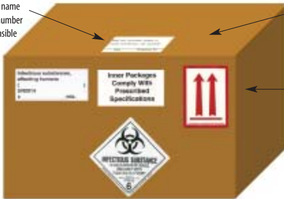
Figure D: Overpack with \geq 50 ml of infectious substance
